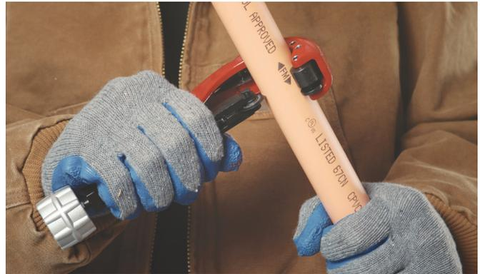
Burrs and filings can prevent proper contact between the pipe and fitting and may put undue stress on the pipe and fitting assembly. For this reason, they must be removed from the outside and inside of the pipe. A chamfering tool or file is suitable for this purpose.
