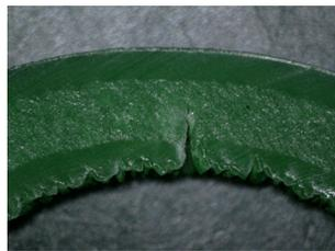
This section of 2-inch pipe recovered from the site is visibly degraded. When new, PP-R pipes are smooth inside and out. However, this pipe's interior had become ridged, with deep cracks nearly extending to its exterior.
